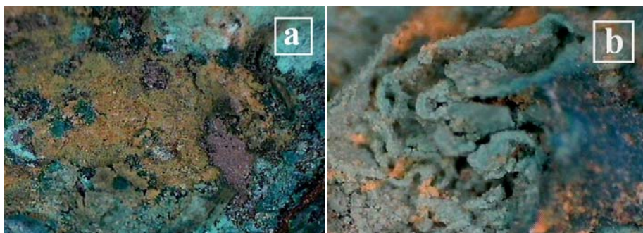
Fig. 2. (a) Optical observation of coin 1, multicolor areas, 65X, (b) Coral reef-shaped corrosion product, 170X.
