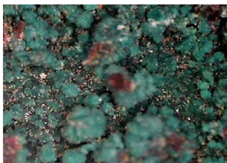
Fig. 3. Optical observation of reniform shape on coin 2, 120X.
