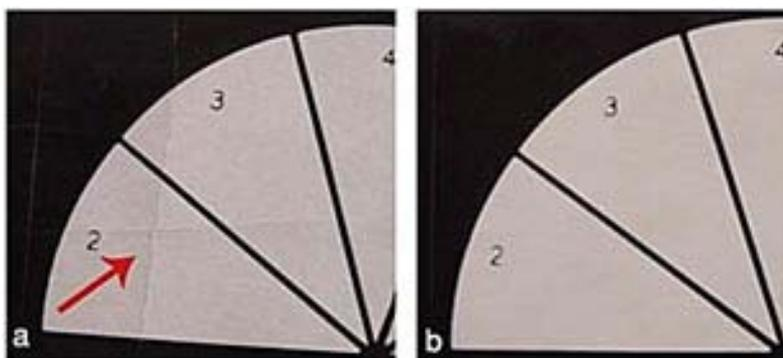
**Fig. 2.** (a): a close-up shot of the crack pattern that has developed after ageing improperly processed sample after ageing at 105°C and 67.5% RH; (b): a properly processed sample aged in the same condition showing no visible signs of cracking.
