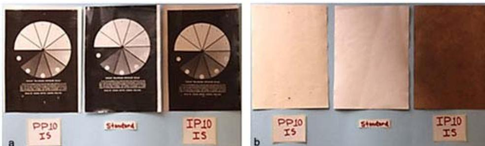
**Fig. 1.** (a): shows the status of sample PP10IS (properly processed) and sample IP10IS (improperly processed samples) after aging. Compared to the control sample, PP10IS they were slightly yellowed, while IP10IS shows severe discoloration. The aging condition is 105°C at 67.5% RH; (b): the verso of the samples showing slight discoloration in the case of the properly processed sample and severe discoloration in the case of the improperly processed sample.
