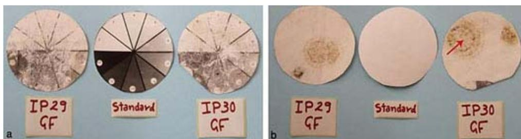
**Fig. 7.** (a): samples IP29GF and IP30GF after exposure to hydrogen sulfide for 15 days at 80%RH. High relative humidity (80%) caused severe degradation of the gelatin binder; (b): the growth of microorganisms on the verso of samples IP29GF and IP30GF after exposure to hydrogen sulfide for 15 days at 80%RH.
