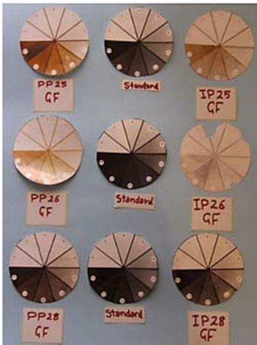
**Fig. 4.** Gas fading test samples after exposure to oxidizing gases. The image silver decay is noticeable in all samples; however, the effect of the gases is much more severe in the case of the improperly processed samples (i.e. IP25GF, IP26GF, and IP28GF compared to PP25GF, PP26GF, and PP28GF respectively).
