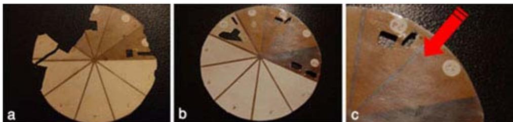
**Fig. 6.** (a): sample IP25GF after exposure to hydrogen peroxide for 10 days showing embrittlement of the paper base but no visible signs of silver mirroring; (b): sample PP25GF showing silver mirroring decay in shadow areas after to the same gas fading test; (c): close-up shot of silver mirroring decay found in sample PP25GF.
