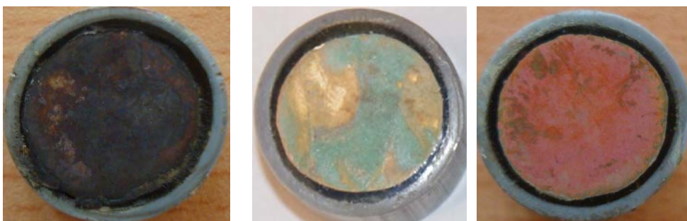
Fig.6. The electrode surfaces after the corrosion test in a solution containing 0.2 g/L \text{Na}_2\text{SO}_4 + 0.2 g/L \text{NaHCO}_3 (pH = 5).
